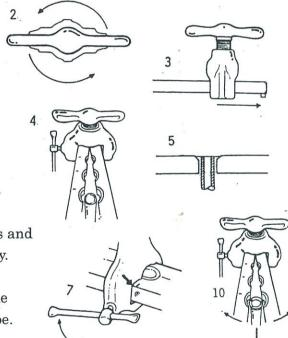
Note: When the clamp bar cannot be open, you can open it by tightening the clamp handle with the body on the end screw.
