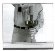
6. Start will a slight pressure on the trigger for slow speed. As more pressure is applied, the drum will spin faster. With the drill running at the desired speed, push the tool gently towards the drain.
