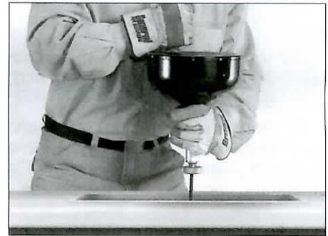
3. Turn the tool clockwise, using a slight forward pressure, until the exposed length of cable enters the drain.
