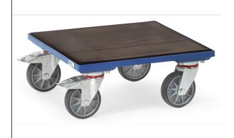
Frame made of angular steel, welded, powder coated, blue RAL 5007. With wooden platform covered with corrugated rubber. 4 swivel castors, wheels with TPE tyres, hubs with precision deep grove ball bearing. 2 swivel castors with wheel locks, according to the European Standard EN 1757-3 (safety of platform trolleys).
