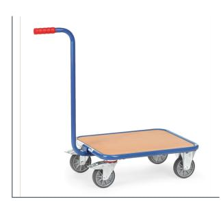
Made of tubular steel welded and powder coated, blue RAL 5007, with wooden platform, handles bolted on. 2 swivel castors and 2 fixed-wheel castors. Wheels with TPE tyres, hubs with precision deep grove ball bearing. Swivel castors with wheel locks, according to the European Standard EN 1757-3 (safety of platform trolleys).
