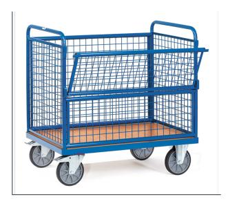
Tubular steel and profile steel welded, powder coated blue RAL 5007. Platform made of derived timber material board, surface beech grain. Wire cage cart with tubular steel superstructure, wire lattice 50 x 50 x 4 mm, welded. Bolted modular version, powder-coated. Useful height: 700 mm. 2 swivel and 2 fixed-wheel castors, TPE tyres, hubs with groove ball bearing. Swivel castors with wheel locks, according to the European Standard EN 1757-3 (safety of platform trolleys).
