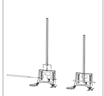
Insert axle through one axle hole in base, through post, and through opposite base axle hole.
