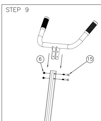
Slide handle onto post and fasten with two locknuts(6) and two bolts(15).
