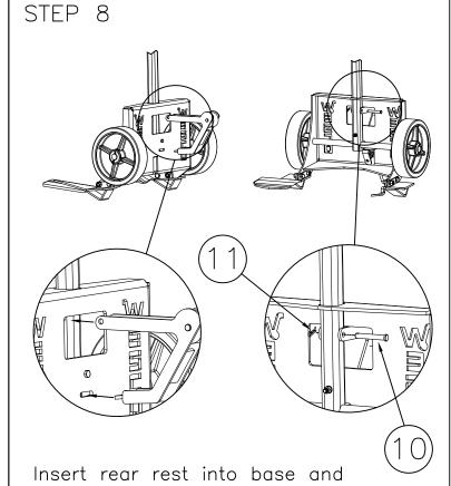
secure with clevis pin(10) and
