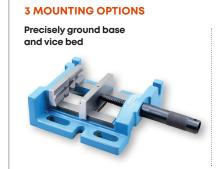
Fully ground side face allows for right angle machining with the same jaw setting. The jaw width acts as jaw height facilitating longer workpieces to be held
