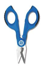
For cutting and stripping of Cu/Al conductors as well as for crimping of terminals from 0.5 to 4 mm<sup>2</sup>. The cutting edges of the scissors are serrated. This achieves a flush cut and the slipping of the cable is prevented.
