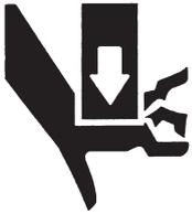
Pinch point hazard: Cutting at high speed and high force can cause severe personal injury. Keep your body parts away from the moving parts of the tool during operation.
