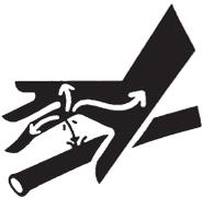
Hydraulic fluid under pressure: Prevent any part of your body from touching or getting close to the hydraulic leak. Escaping fluid under pressure can cause severe injury or death. In case of injury results from any fluid leakage, get medical attention immediately to avoid serious bodily harm.
