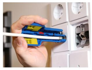
Working with WEICON Stripping tools is only permitted with potential free wires and conductions
