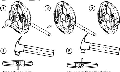
Align hole and drive from back side to start pin
