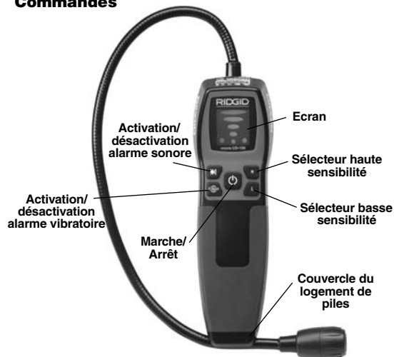
Figure 2 – Composants du micro CD-100
