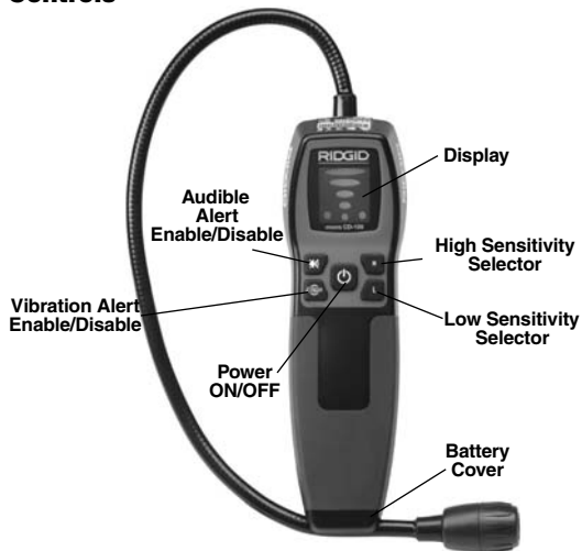
Figure 2 – micro CD-100 Parts
