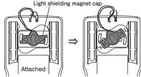
Turn the light shielding magnet cap counterclockwise to detach.
