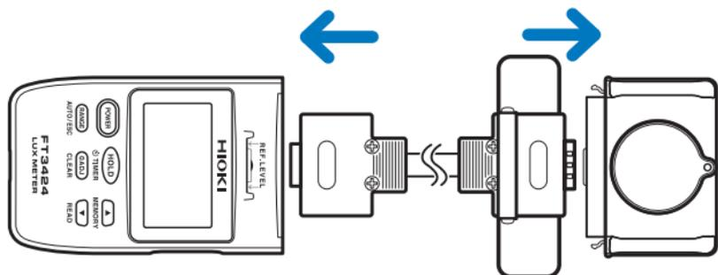
Do not separate and connect the display unit and the sensor unit while the instrument power is on.
