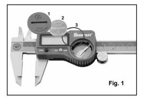
First, unscrew and remove the battery cover (1) by turning it to the left ¼ turn. Remove the old battery. Next, position the rubber "O" ring (3) correctly in the bottom of the battery compartment before inserting the new battery (2) negative side (-) down. Then, re-install the battery cover (1) and lock it into position by giving it a ¼ turn to the right.
