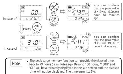
• Pressing the [Air Adjustment] switch while the detector is off can display the last peak value. However, turning on the detector will reset the peak value to 0ppm (21.0% for oxygen
