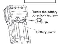
(4) Install the battery cover. Rotate the battery cover lock (screw) clockwise with a Phillips screwdriver. (Recommended torque: 22 cN·m)
