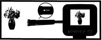
7. To ensure the camera shows an accurate angle on the home screen after bending, adjust the arm by lightly twisting it until the TOP mark is aligned to the top of the CART body.
