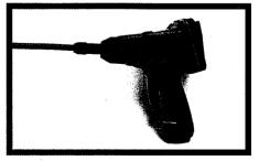
6. To hold the claws out of the camera view when searching for an object, use the handle clip to hold the trigger until the claw is needed.
