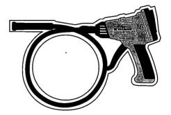
2. When bending, always keep the radius more than 7 in., or the claw may not function properly. NEVER bend the arm past 90 degrees, or the claw may not function properly.
