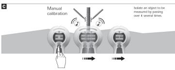
Tip 1: The position between the two markings is the mid-point of the metal object. Through the high measuring sensitivity, thick metal objects appear broader than they are in real life. Therefore move the device over the newly found object as shown in Image B. The device is calibrated automatically during this process. Manual calibration should be performed near the place found last as shown in Image C. Repeat this step as needed.
