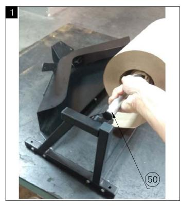
Insert 50 support tube into core of paper roll. Position the paper roll to the dispenser as shown.
