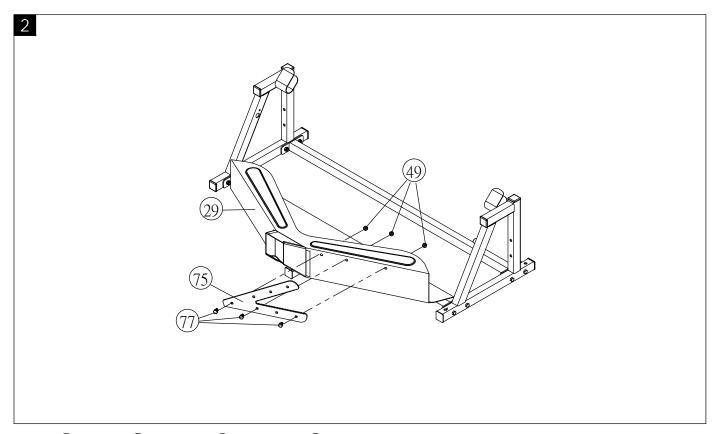
$\label{prop:control} \textit{Fasten} \ \ \, \boxed{75} \textit{cutter to} \ \ \, \boxed{9} \textit{chute with} \ \ \, \boxed{77} \textit{screws and} \ \ \, \boxed{49} \textit{nylon nuts.}$
