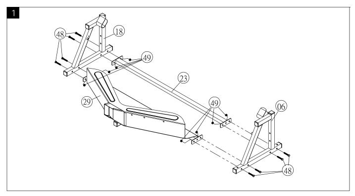
Install@chute and@bridge assembly to@left frame assembly and@right frame assembly with@screws and@nylon nuts.
