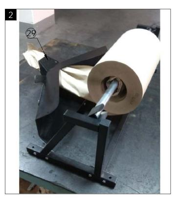
Feed paper under the paper roll. Also feed paper through (29) chute.
