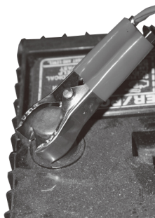
FIGURE 11 Red Positive (+) to Battery
