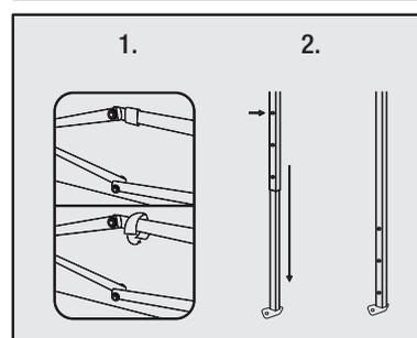
(3.) Depress snap button or pull the pin on the slider at the corner bracket to disengage the frame and allow it to close.
