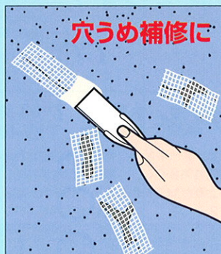
ひび割れ補修に
