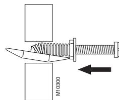
Drill a hole in accordance with the table. Attach the toggle in the guide collar and install.
