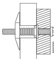
Remove the screw. Mount the fixture.
