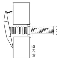
Push screw until spring-loaded bar flips over.
