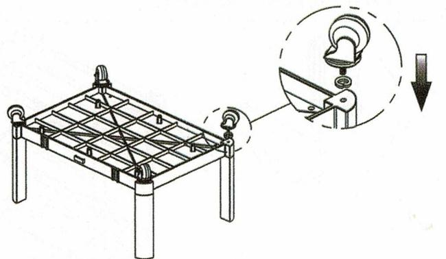
4. Install wheels and tie up by spanner.
