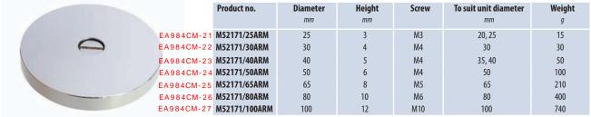
To achieve the optimum pull force 100% contact area must be achieved using the recommended armature plate. The force will be affected if other material specifications, thicknesses and surfaces are used, or if the armature fails to make positive contact over the full diameter of the face of the magnet. Where misalignment is likely to be an issue we recommend that an oversized armature plate is used to ensure 100% full contact, this however will reduce the stated pull force by approximately 10%.
